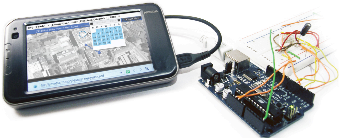
Figure 1. A Nokia N810 Internet tablet displaying the Envismo mobile interface for mapping energy usage data. An attached Arduino microcontroller and environmental sensors provide supplemental environmental data.
